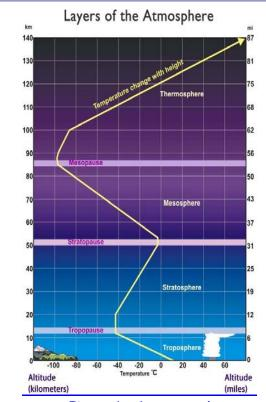
Figure 1 - Layers and temperatures of the atmosphere.
